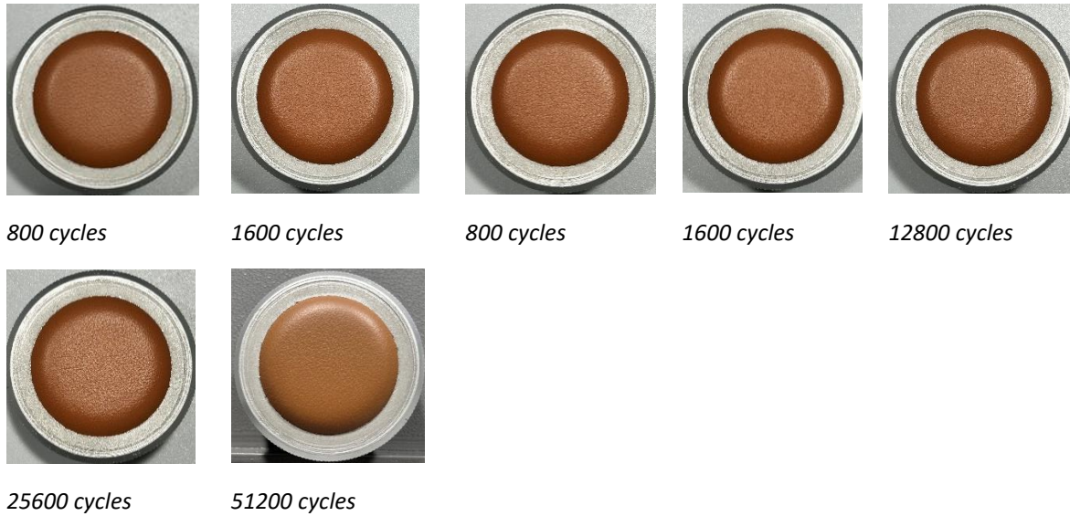
Fig. 16 – Leather for iPhone casing Martindale abrasion test
